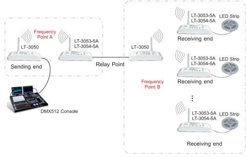
5.3 Extend the communication distance by boost antenna:
